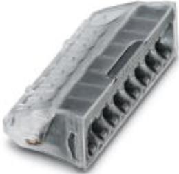
8-pos. socket terminal block with spring-cage connection, for toolless wiring with push-in connection method, for one and multi-strand conductors with a cross section of 0.5 to 2.5 mm<sup>2</sup>, insulation housing transparent.
