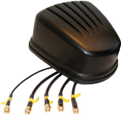
Pulse Panther Series is a roof mount antenna with five connectors, two each for LTE and WLAN and one for GNSS (GPS and GLONASS). This compact, aesthetically pleasing solution combines ideal radiation performance for today's demanding propagation environments with optimum isolation characteristics ensuring highest data rates possible.
