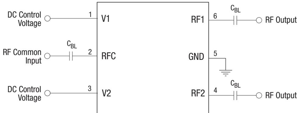
$C_{BL} = 47 \text{ pF}$  for >1 GHz operation. Increase value for lower frequency operation.
