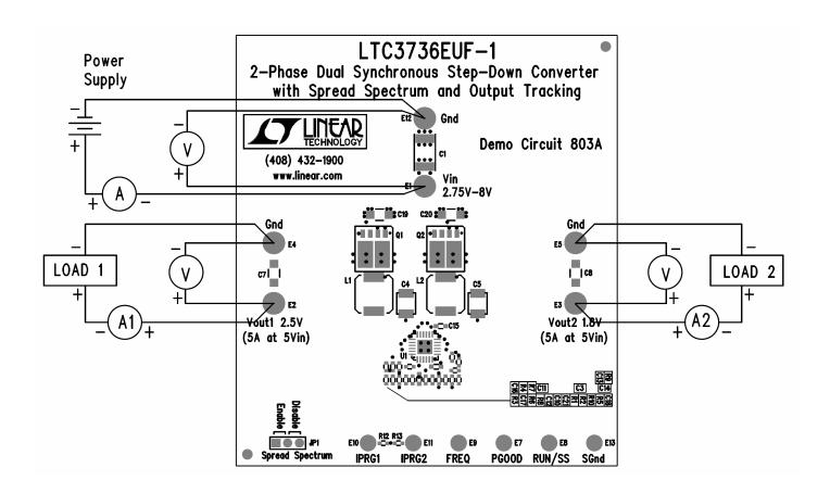
Figure 1. Proper Measurement Equipment Setup
