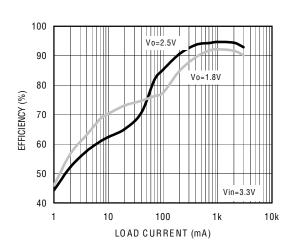
Figure 2. Efficiency vs load current (550kHz)
