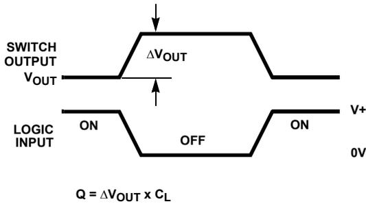
$$Q = \Delta V_{OUT} \times C_L$$
