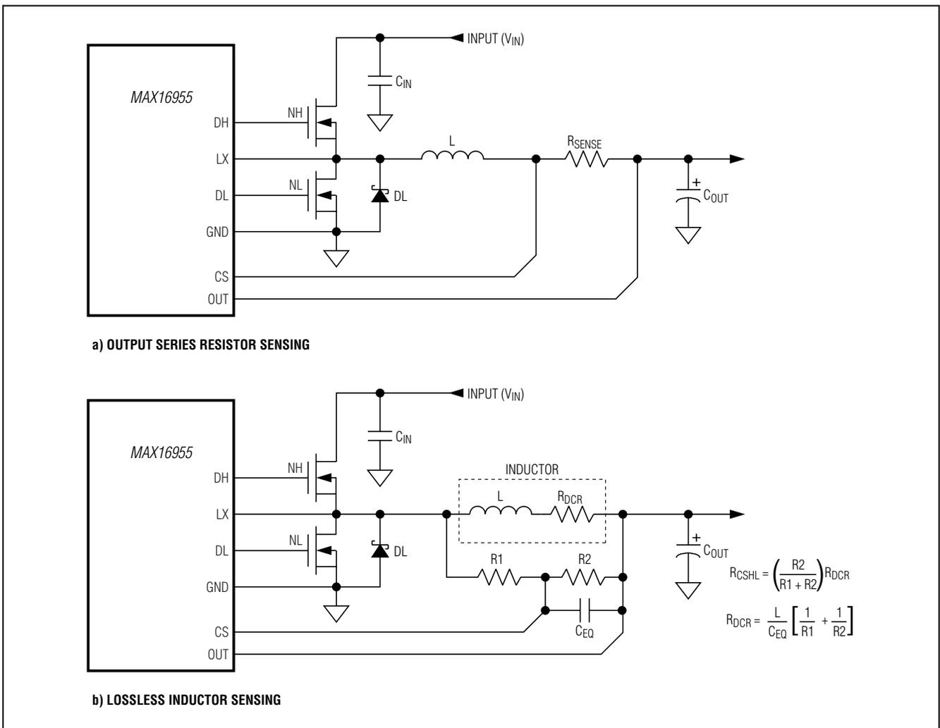
Figure 4. Current-Sense Configurations
