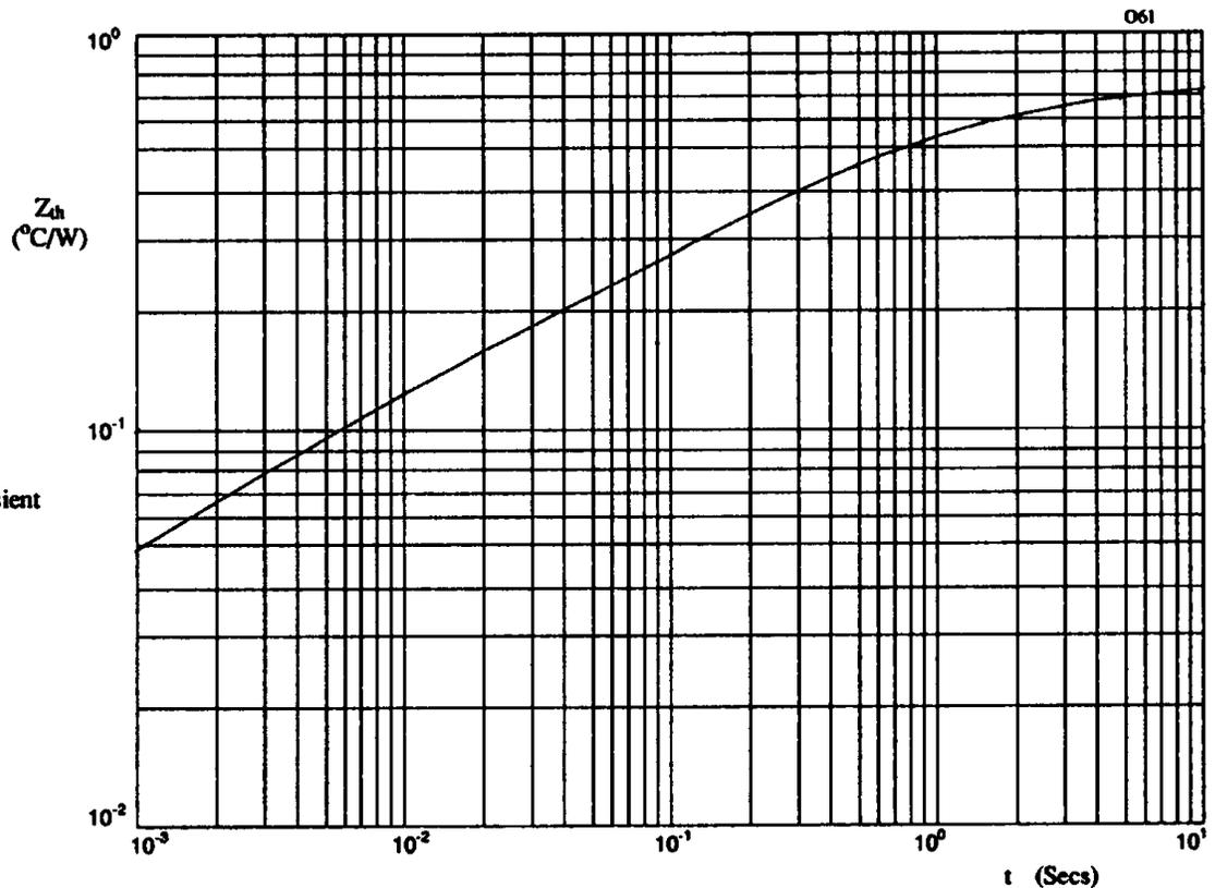
Figure 1. Typical transient thermal impedance characteristic.
