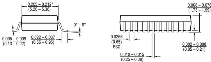
\*THESE DIMENSIONS DO NOT INCLUDE MOLD FLASH OR PROTRUSIONS. MOLD FLASH OR PROTRUSIONS SHALL NOT EXCEED 0.006 INCH (0.15mm).
