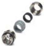
EMC screw connection up to 5 bar, thread length: 15 mm, cable diameter: 19.0 - 28.0 mm, WAF 45, screw connection: M40
