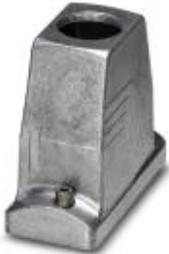
HEAVYCON ADVANCE sleeve housing B16, with high-grade steel screw locking (hexagonal socket-head), salt water resistant aluminum, height 100 mm, with 1xM40 thread, straight cable outlet, without surface; conductive seal (EMC properties)
