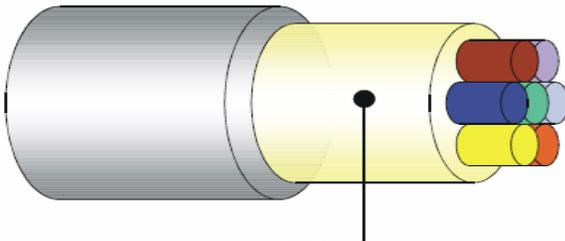
**Use Aluminum foil to cover those wires, for isolating the external noise.**
