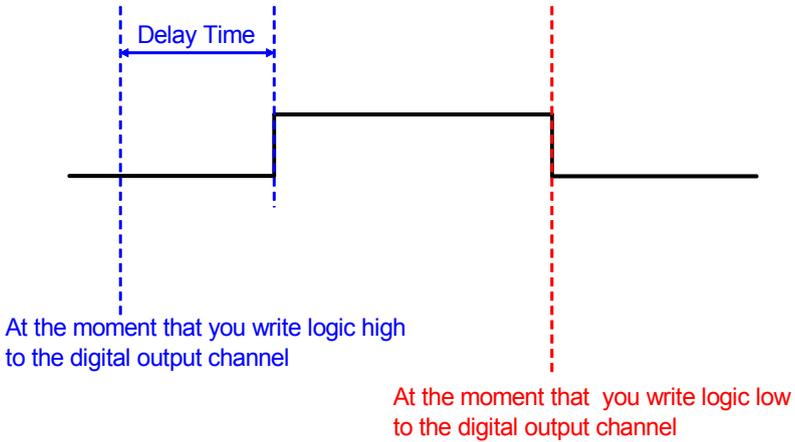
**Figure 5.16: Low to High Delay Output Mode**
