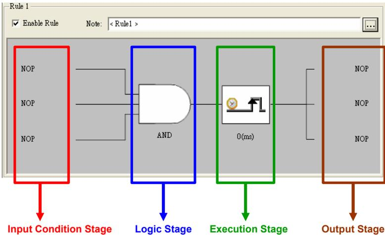
*Figure 7.2: Four Stages for One Logic Rule*
