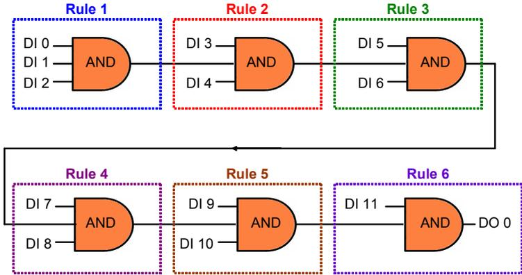
**Figure 7.28: GCL Logic for 12 DI to 1 DO**
