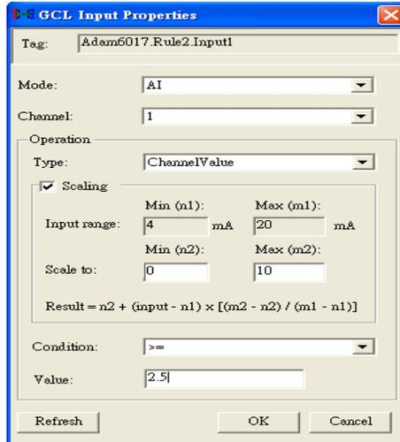
*Figure 7.5: Scaling Function of Analog Input Mode*
