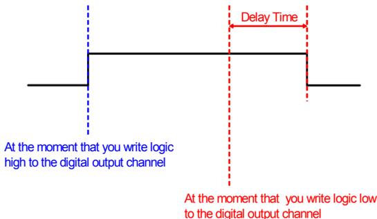
**Figure 5.17: High to Low Delay Output Mode**
