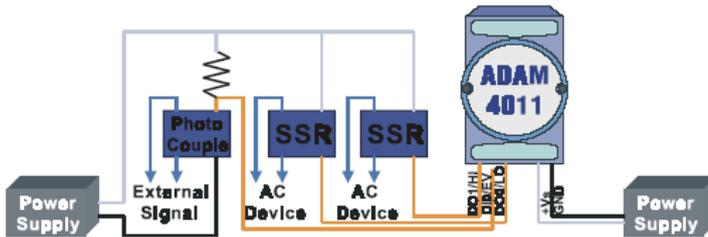
**Separate Load and Device power.
