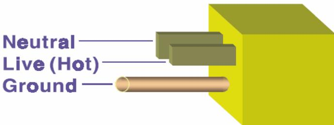
Ground-pin is longer than others, for first contact to power system and noise bypass.
