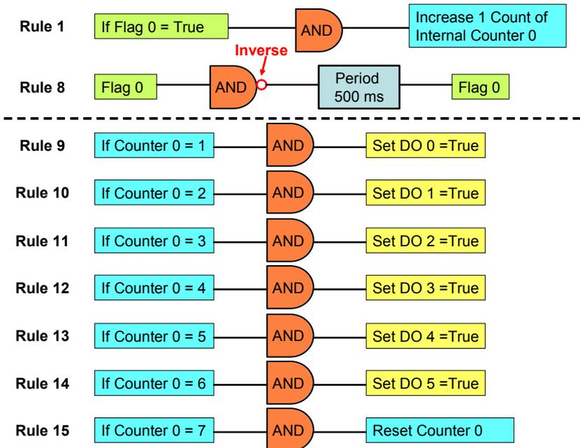
**Figure 7.38: GCL Logic for Sequence Control**
