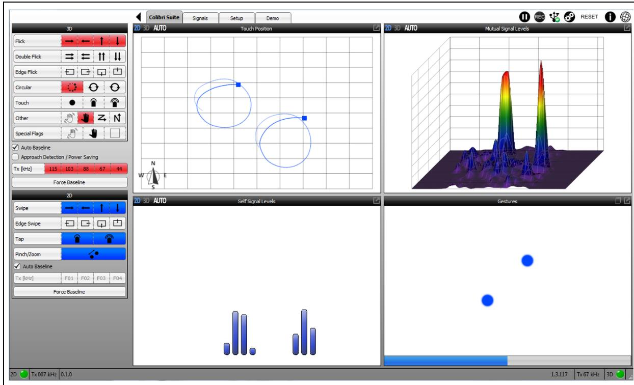
11. Use your hand to swipe left to right over the 2D/3D sensor module. Verify that the red gesture arrows follow your movements in the bottom right Gestures window. The hand distance should be ~10 cm (up to 20 cm) above the sensor. Always check that the desired gesture is actually activated in the 2D and/or 3D overview on the left side of the screen.
