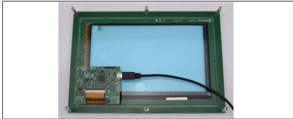
3. Carefully turn the assembled hardware over and lay on a flat table surface. The six stand-offs support the hardware, creating a flat level touch surface.
