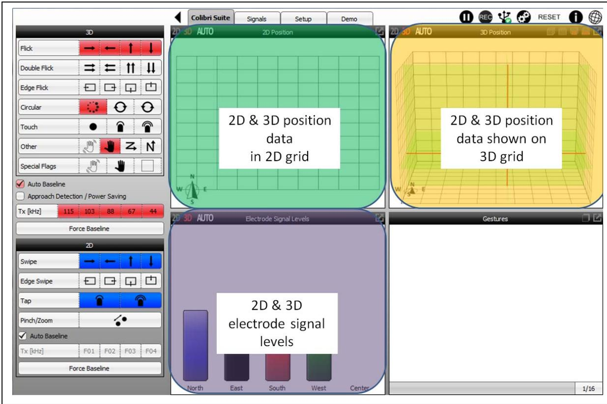
10. Use your finger(s) to draw a circle on the touch screen surface area inside the black borders and verify that the points in the top center 2D Measurement window follow your circular motion.
