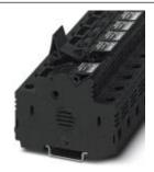
Fuse modular terminal block, with light indicator, Connection method: Screw connection, Cross section: 1.5 mm²- 25 mm², AWG: 16 - 4, Nominal current: 32 A, Nominal voltage: 690 V, Width: 18 mm, Fuse type: Cartridge fuse insert 10.3 x 38 mm, Fuse type: Glass, Mounting type: NS 35/7,5, NS 35/15, Color: black/red
