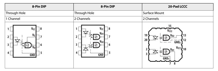
**NOTE** All DIP devices have common  $V_{CC}$  and ground. LCCC (leadless ceramic chip carrier) package has isolated channels with separate  $V_{CC}$  and ground connections. All diagrams are top view.
