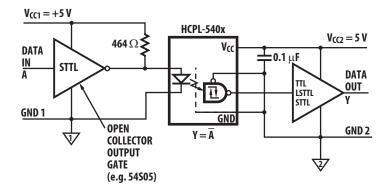
Figure 15 Recommended HCPL-543x and HCPL-643x Interface Circuit
