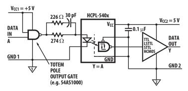
Figure 14 Alternative HCPL-540x Interface Circuit
