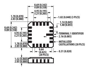
Note: Dimensions in millimeters (inches). Solder thickness 0.127 (0.005) max.
