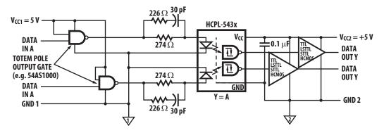
Figure 16 Alternative HCPL-543x and HCPL-643x Interface Circuit
