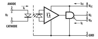
Note: Enable pin 7. An external  $0.01-\mu F$  to  $0.1-\mu F$  bypass capacitor must be connected between  $V_{CC}$  and ground for each package type.
