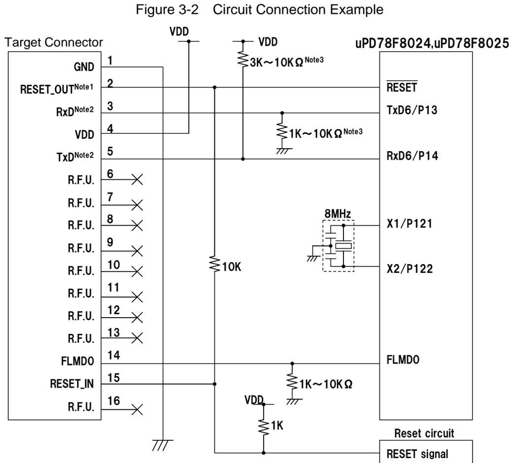
Note1. This connection is designed assuming that the RESET signal is output from an N-ch open-drain buffer (output resistance: 100Ω or less).
