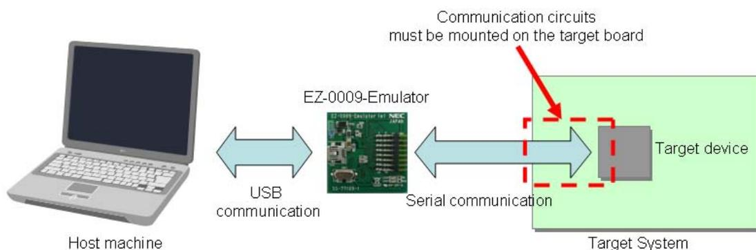
\* Communication circuits are mounted on Target board (QB-78F8025-TB)
