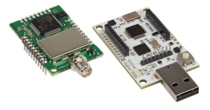
MultiConnect® mDot<sup>TM</sup> with Micro Developer Kit MTMDK-ST-MDOT Quick Start
