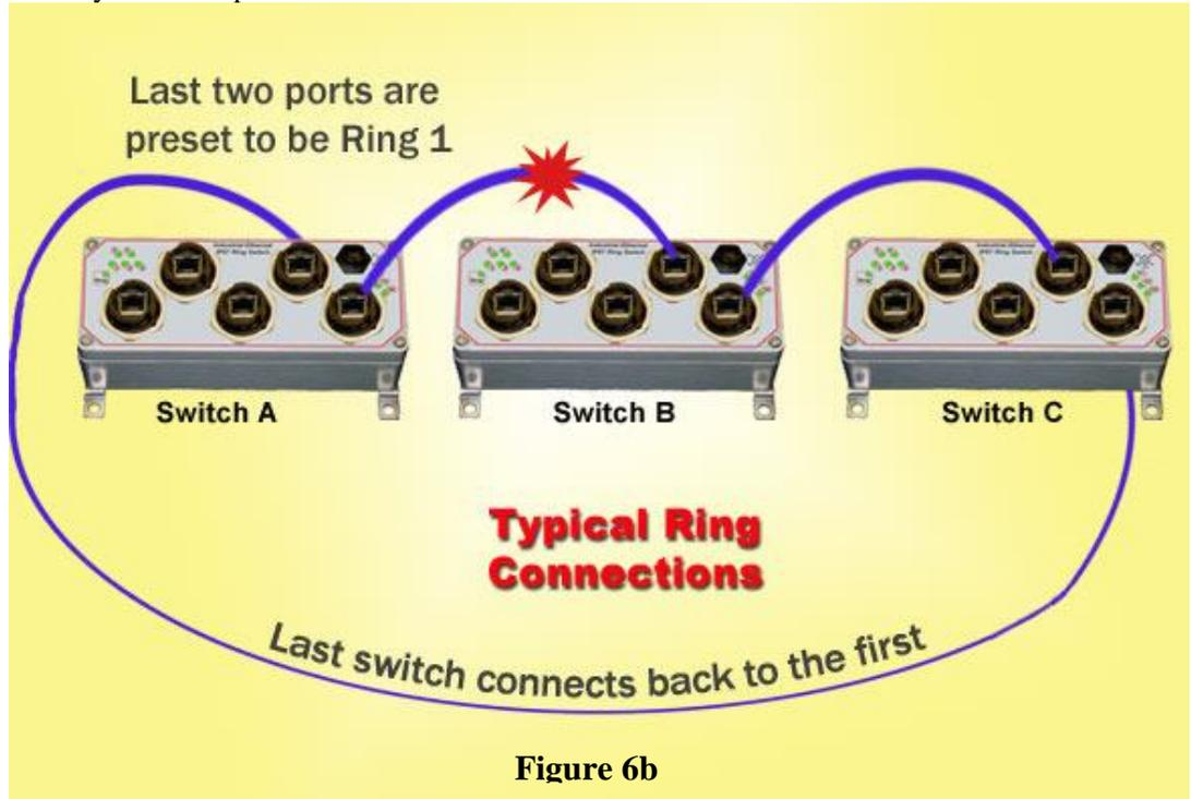
With the break indicated above, we would expect these values from the Modbus registers of each switch:
