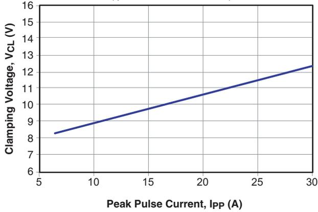
**Clamping Voltage vs. Current**
