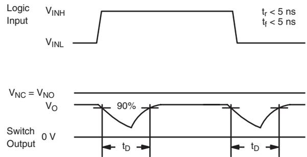
Figure 2. Break-Before-Make Interval
