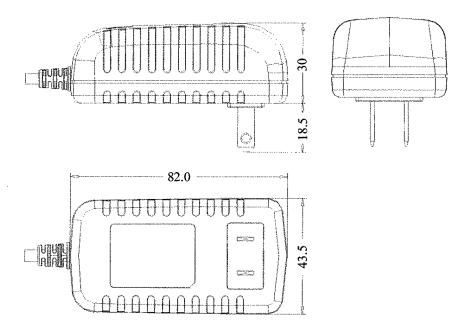
NOTE:1. Case cover & chassis material: PC/ABS (UL94V-1) BLACK
