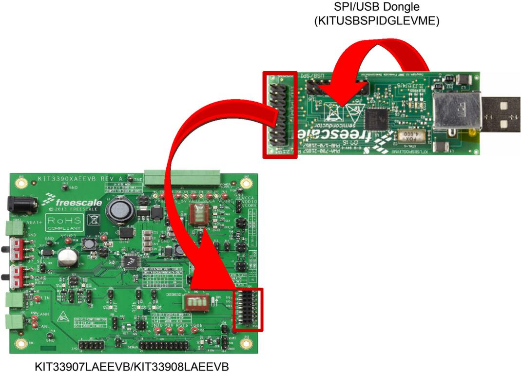
Figure 7. Connecting KITUSBSPIDGLEVME to the Evaluation Board
