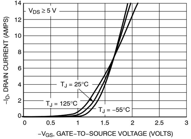
**Figure 2. Transfer Characteristics**
