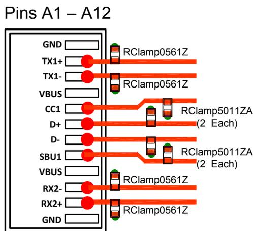
Figure 2 - USB Type-C Bottom Layer Protection Example
