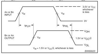
**Waveform 1. Input to Output Propagation Delays**
