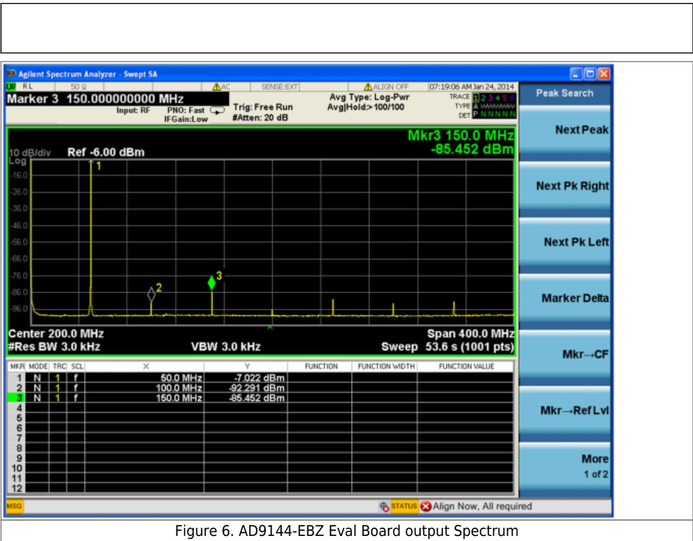
Figure 6. AD9144-EBZ Eval Board output Spectrum
