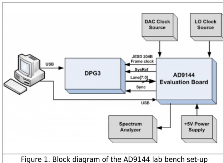
Figure 1. Block diagram of the AD9144 lab bench set-up
