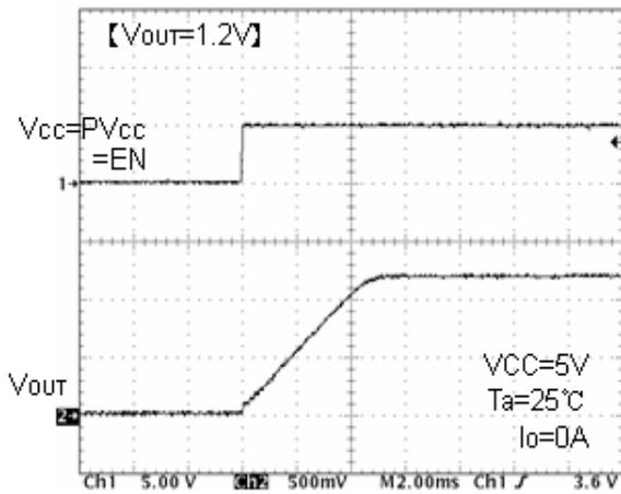
Fig.14 Soft start waveform
