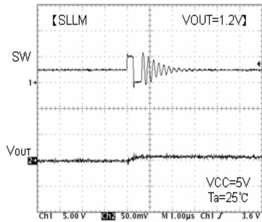
Fig.15 SW waveform I<sub>o</sub>=10mA
