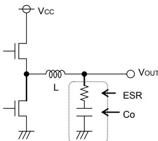
Fig.29 Output capacitor
