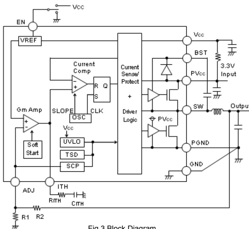
Fig.3 Block Diagram
