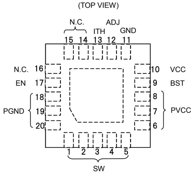
Fig.2 Pin Configuration
