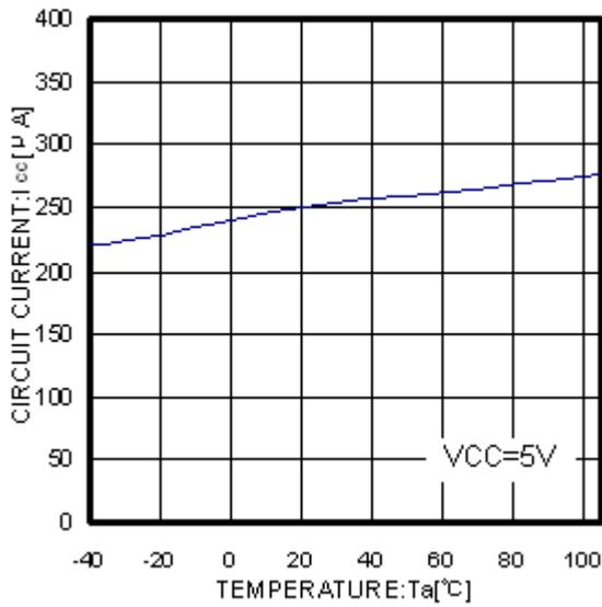
Fig.12 T<sub>a</sub> - I<sub>cc</sub>
