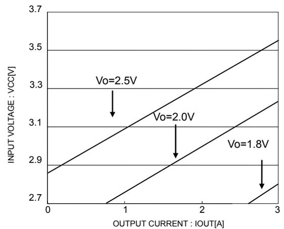
Fig.35 minimum input voltage in each output voltage
