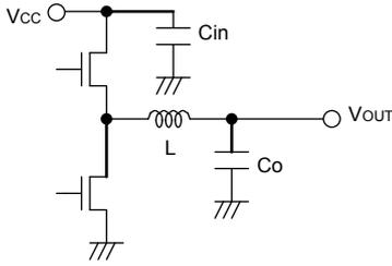
Fig.30 Input capacitor
