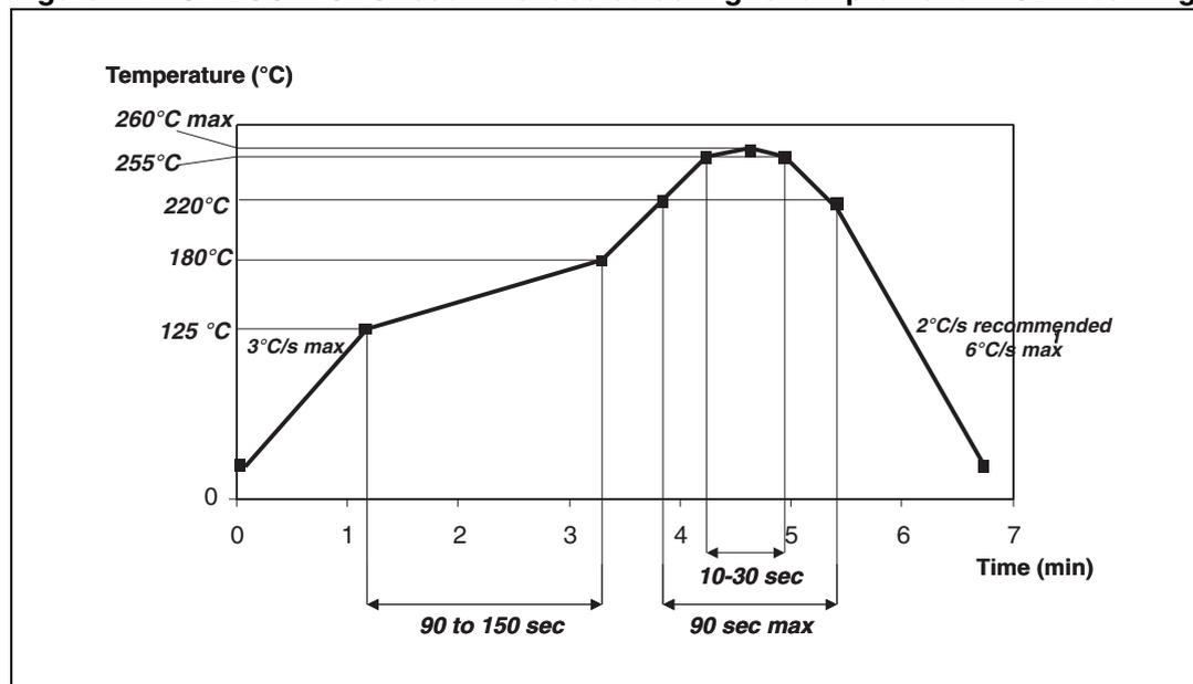
Dwell time in the soldering zone (with temperature higher than 220 °C) has to be kept as short as possible to prevent component and substrate damages. Peak temperature must not exceed 260 °C. Controlled atmosphere (N<sub>2</sub> or N<sub>2</sub>H<sub>2</sub>) is recommended during the whole reflow, especially above 150 °C.
