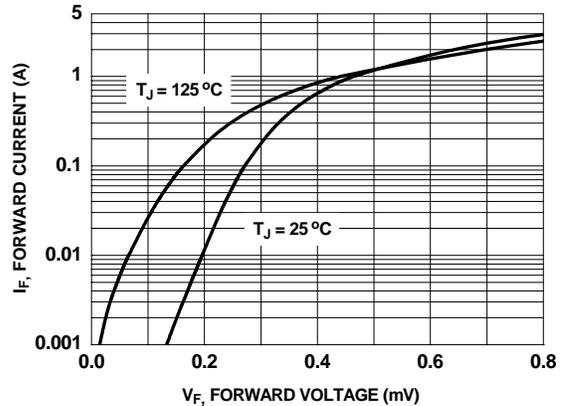
**Figure 12. Schottky Diode Forward Voltage**
