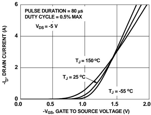
Figure 5. Transfer Characteristics
