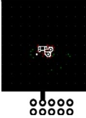
a. 90 °C/W when mounted on a 1 in<sup>2</sup> pad of 2 oz copper.
