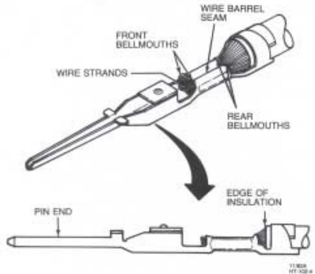
Figure 4. Correctly Crimped Terminal
