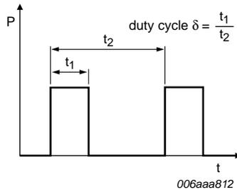
Fig 17. Duty cycle definition
