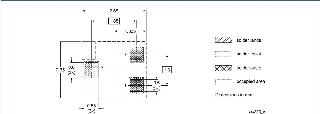
Fig 19. Reflow soldering footprint for SOT323 (SC-70)
