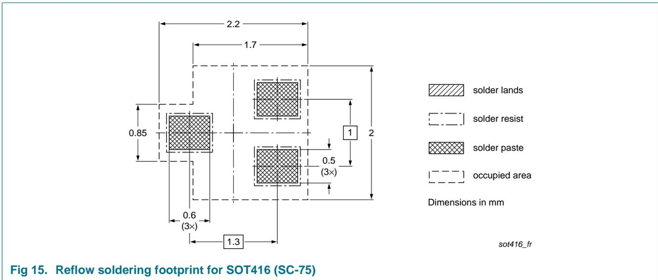
Fig 15. Reflow soldering footprint for SOT416 (SC-75)
