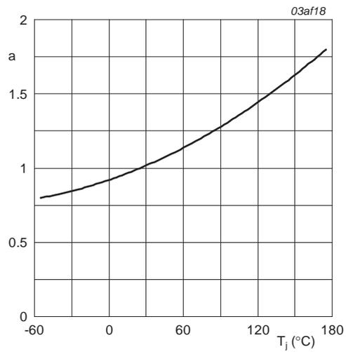
$$a = \frac{R_{DS(on)}}{R_{DS(on)@25^\circ\text{C}}}$$
