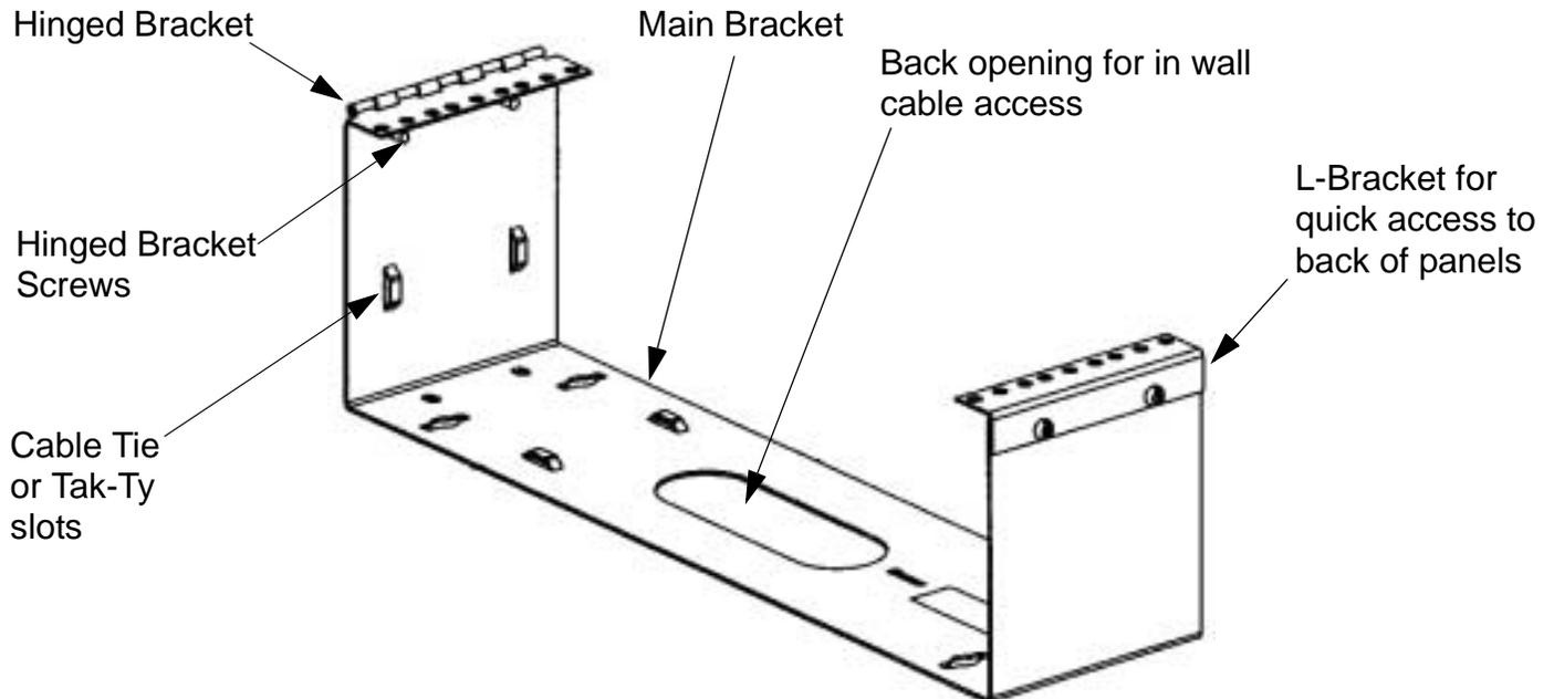
NOTE: WBHE models are packaged without hinges or L-brackets installed. Mount hinges and L-brackets on the outside of the Main Bracket as shown, using the supplied #12-24 screws and pem nuts. Make certain the pem nuts are facing the back of the Main Bracket.
