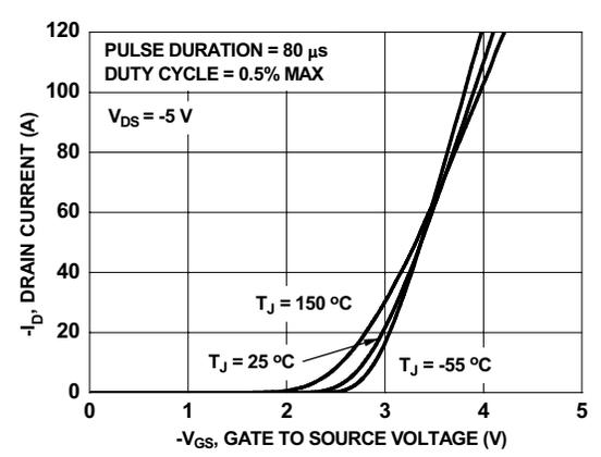
**Figure 5. Transfer Characteristics**
