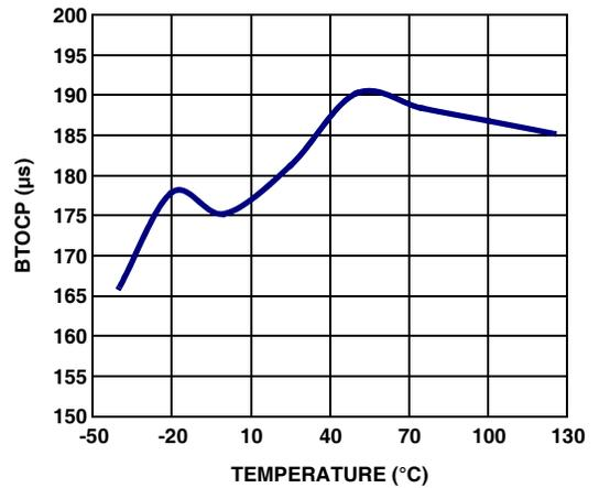
FIGURE 15. OVERCURRENT PROTECTION BLANKING TIME vs TEMPERATURE
