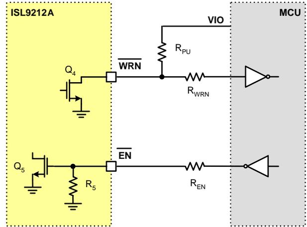
FIGURE 24. DIGITAL SIGNAL INTERFACE BETWEEN ISL9212A AND MCU
