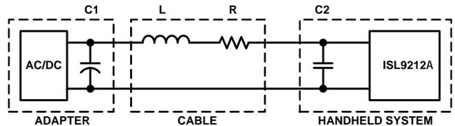
FIGURE 25. EQUIVALENT CIRCUIT FOR THE ISL9212A INPUT
