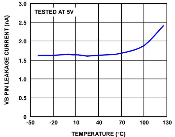
FIGURE 19. VB PIN LEAKAGE CURRENT vs TEMPERATURE
