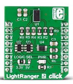
**LightRanger 2 click** carries VL53L0X IC from STMicroelectronics, the word's smallest Time-of-Flight ranging and gesture detector sensor. The click is designed to run on either 3.3V or 5V power supply. LightRanger 2 click communicates with the target microcontroller over I2C interface and the following pins on the mikroBUS<sup>TM</sup> line: RST, INT.
