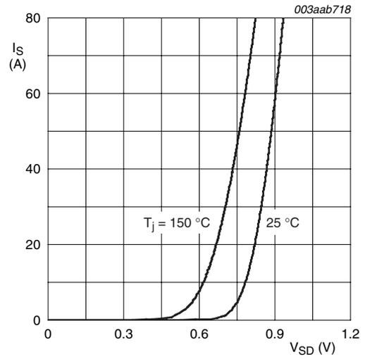
$T_j = 25\text{ °C and }150\text{ °C}; V_{GS} = 0V$
