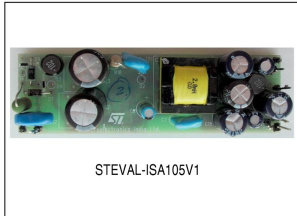
feedback. This eliminates the need for the optocoupler, the secondary voltage reference, as well as the current sensor, while still maintaining quite accurate regulation.
