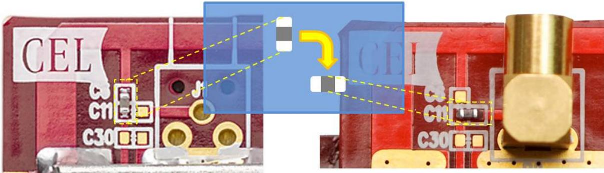
**Figure 41 – Diagram, External Antenna Capacitor Change**
