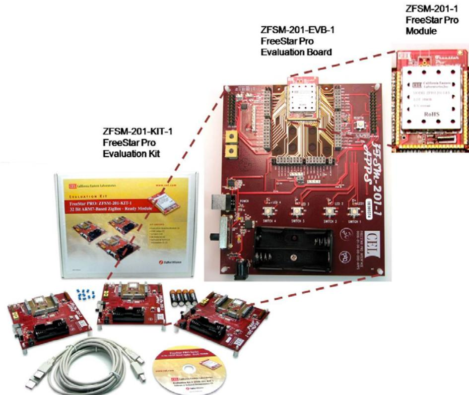
The main component in the Evaluation Kit is the **ZFSM201-EVB-1** FreeStar Pro Evaluation Board. The board serves as an interface, evaluation and development tool enabling the user to demonstrate, and evaluate the capabilities of the CEL **ZFSM-201-1**, FreeStar Pro Module. At the heart of the CEL **ZFSM-201-1** is the Freescale **MC13224V** Platform-in-Package (PiP) transceiver, a 32-bit ARM-based ZigBee radio module and a third-generation 2.4GHz IEEE® 802.15.4 platform.
