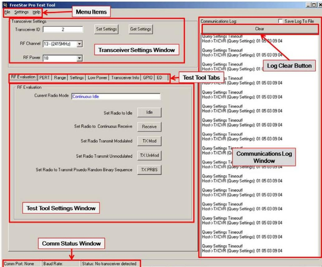
Figure 3 – Screen, FreeStar Pro Test Tool (Opening)
