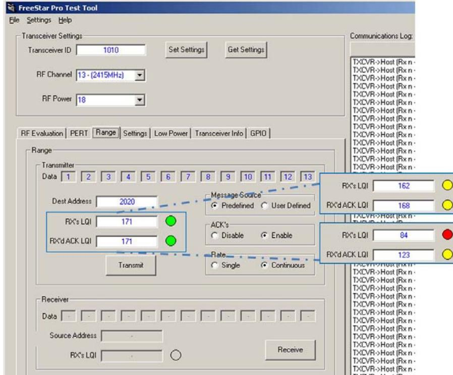
Figure 24 – Screen, Test Tool – Range TX
