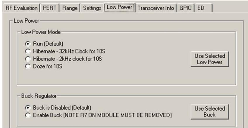
Figure 16 – Screen, Test Tool – Low Power Mode/Buck Regulator
