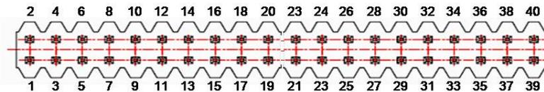
**Figure 2 – Pin numbering for the 40-pin Jumper Connectors (J13, J14 and J15)**
