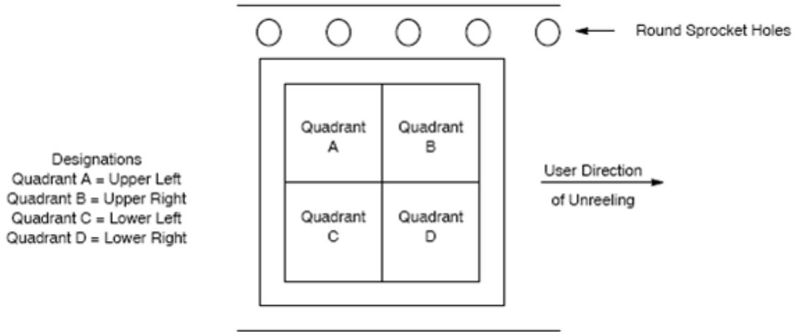
Figure 13. Tape and Reel Pin 1 Quadrant Orientation
