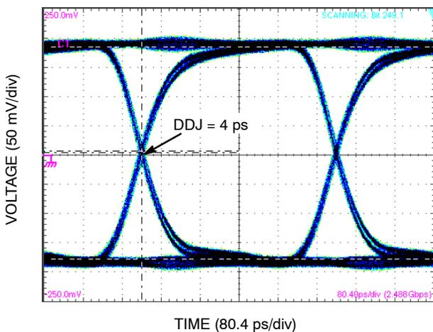
**Figure 7. Typical Output Waveform at 2.488 Gb/s with PRBS 2<sup>23</sup>-1 (Input Signal DDJ = 12 ps)**
