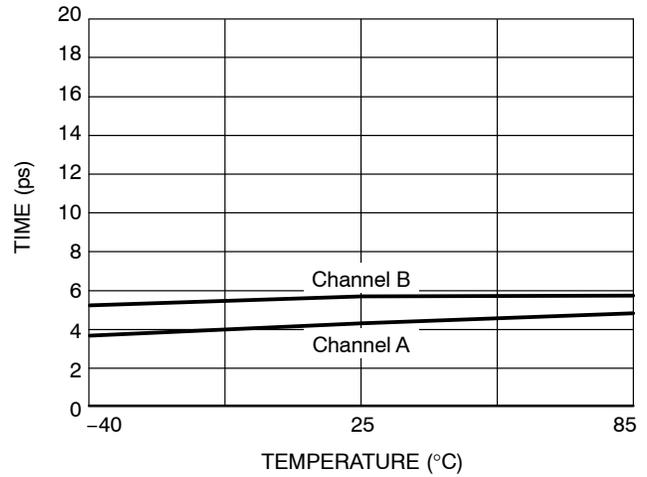
**Figure 4. Within-Device Skew vs. Temperature at  $V_{CC} = 3.3 V$**
