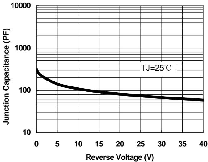
Fig.1-Typical Junction Capacitance
