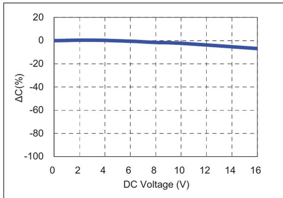
4) Bias TCC characteristics (Agilent 4284A, 1kHz, 1.0Vrms, 8Vdc)
