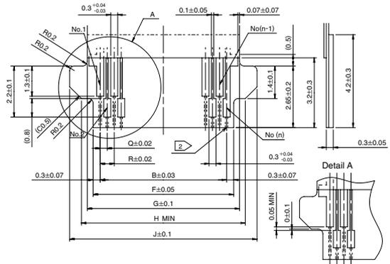
Note ① : Conductor width shall be 0.1±0.05 if FPC has plating bars.
