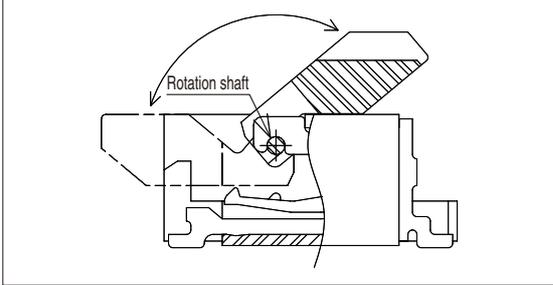
Be careful not to apply excessive force when operating the actuator from the open position (before the FPC has been inserted).
