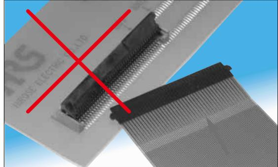
Properly insert the FPC positioning tabs into the corresponding areas on both sides of the insulator body.
