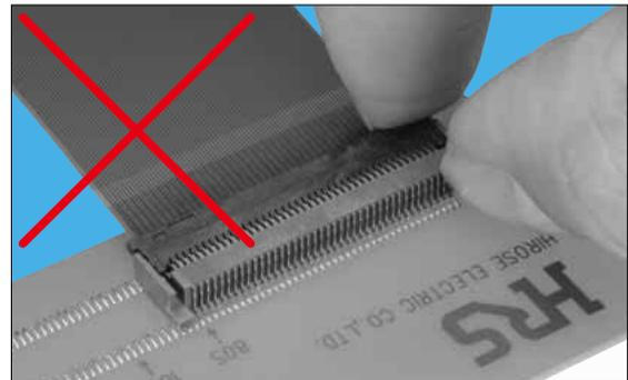
**⑤ Forces to the FPC after insertion and closing of the actuator.**
