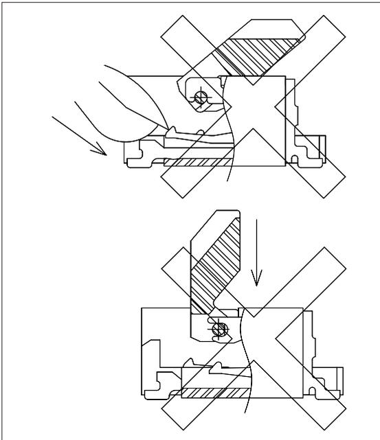
During the closing of the actuator do not pull up or push on it directly down.
