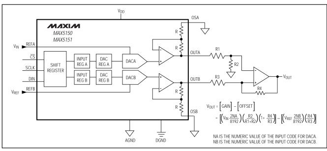
Figure 14. Digital Control of Gain and Offset
