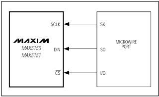
Figure 2. Connections for Microwire
