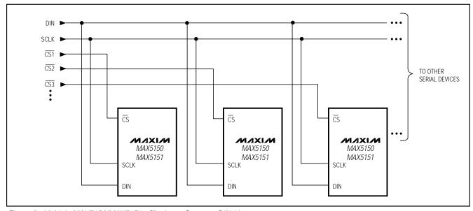
Figure 8. Multiple MAX5150/MAX5151s Sharing a Common DIN Line
