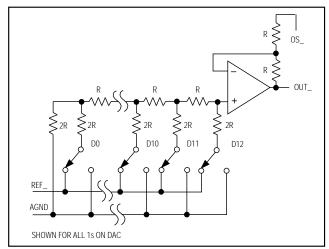
Figure 1. Simplified DAC Circuit Diagram
