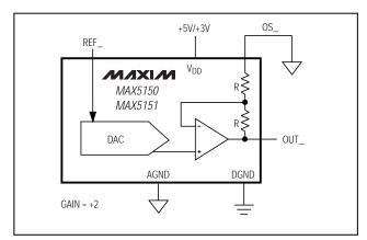
Figure 9. Unipolar Output Circuit (Rail-to-Rail)
