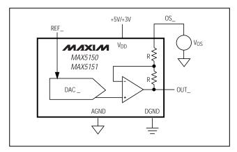
Figure 10. Setting OS\_ for Output Offset
