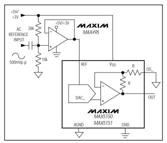
Figure 12. AC Reference Input Circuit
