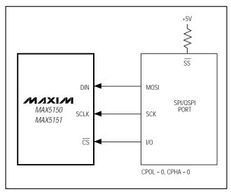
Figure 3. Connections for SPI/QSPI
