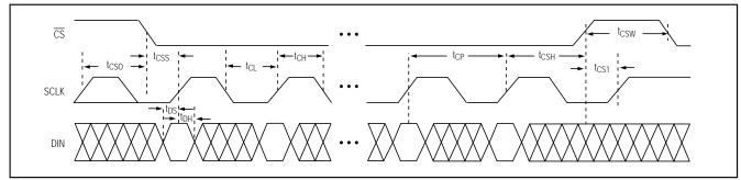
Figure 6. Detailed Serial-Interface Timing Diagram
