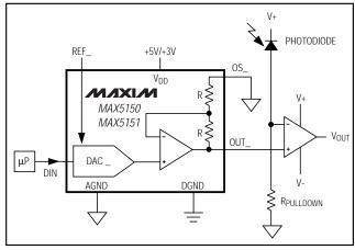
Figure 13. Digital Calibration
