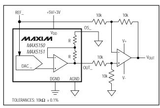
Figure 11. Bipolar Output Circuit
