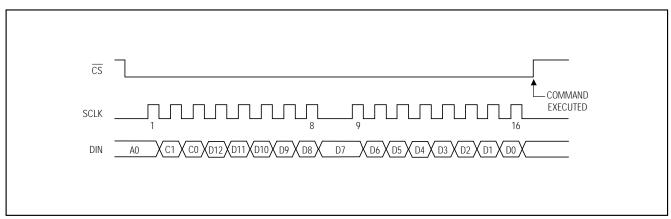
Figure 5. Serial-Interface Timing Diagram
