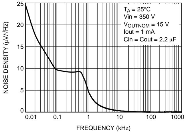
Figure 6. Output Voltage Noise Density vs. Frequency
