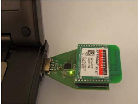
**Note:** *The Portal software does not need to be installed for the SNAPstick to draw power from a PC's USB port.*
