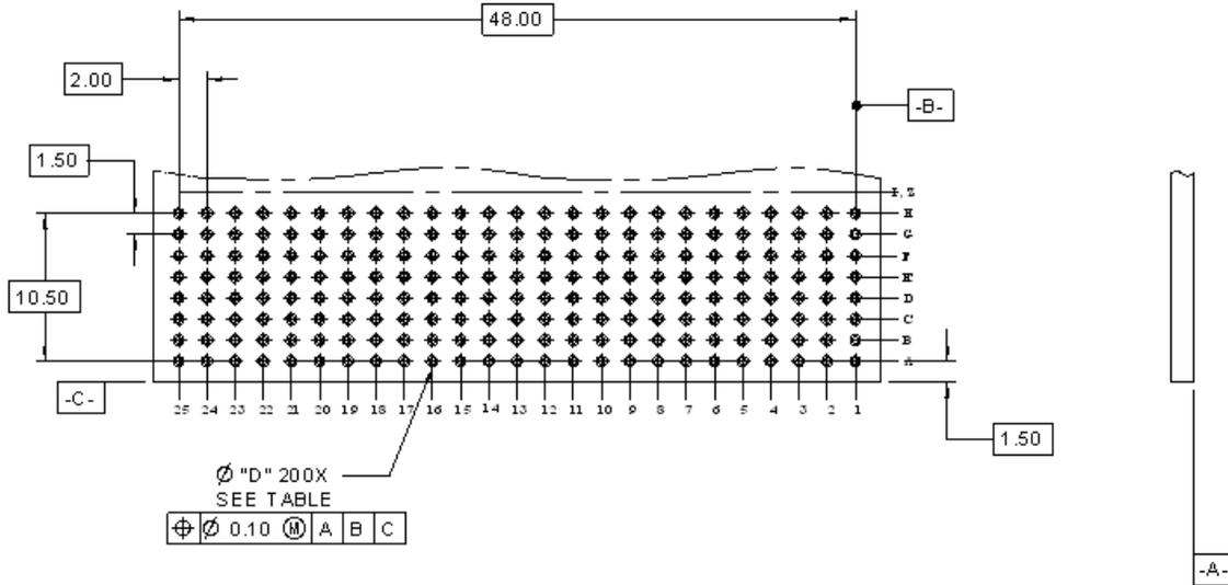
**Recommended PCB Hole Mounting Pattern**
