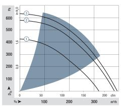
Air performance measured according to: ISO 5801. Installation category A, with ebm-papst inlet ring without contact protection.
