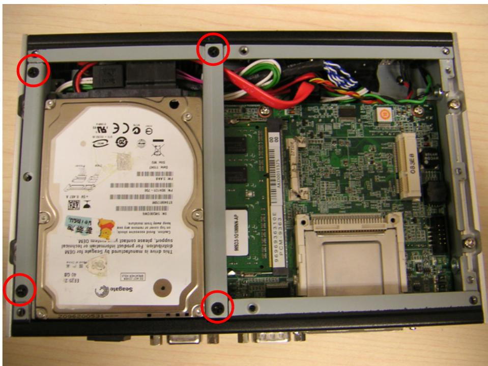
**Figure 2.21** Secure HDD
