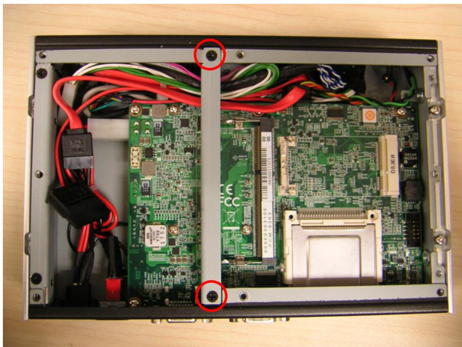
Figure 2.17 Unscrew the screws of the right HDD bracket
