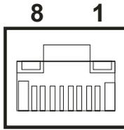
Figure 2.5 Ethernet Connector
