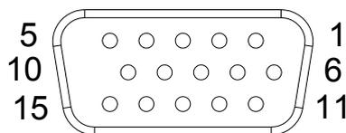
Figure 2.6 VGA Connector
