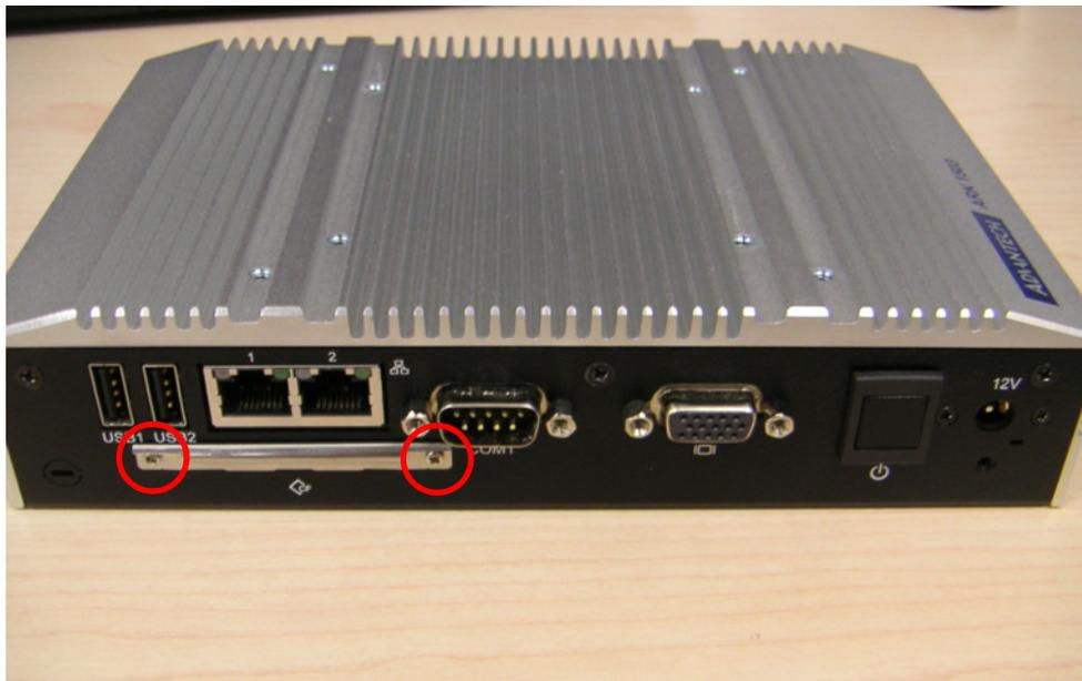
**Figure 2.12 Remove the CF door screws**
