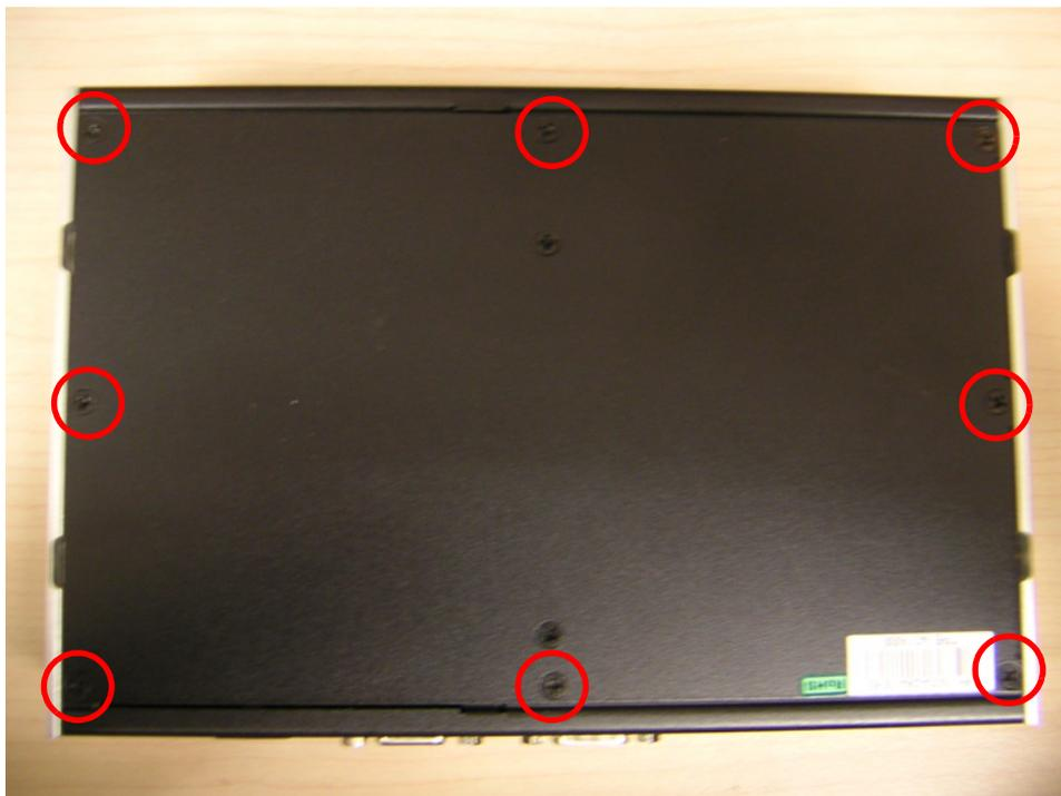
Figure 2.16 Unscrew the screws of bottom cover
