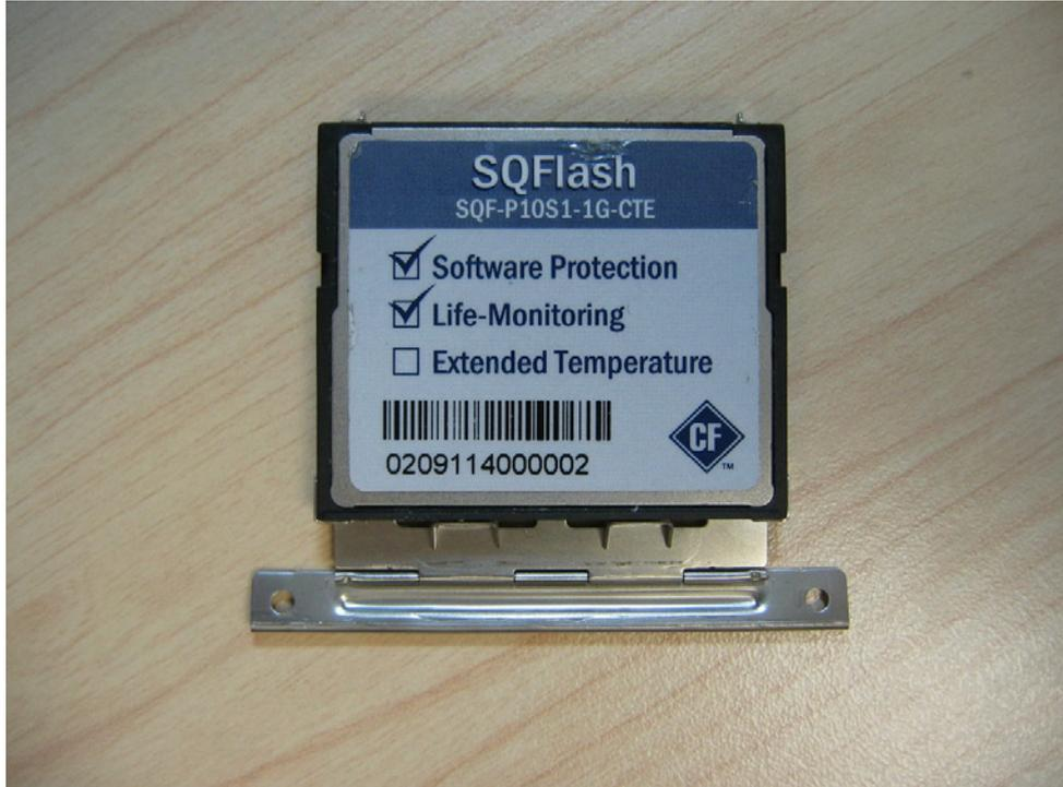
**Figure 2.15 Put CF on to the CF tray**
