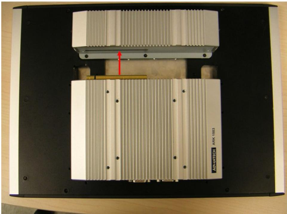
3. Secure the four screws to fix the ARK-1503P to the ITM panel. (The screws are in the accessory box of ITM series products.)
