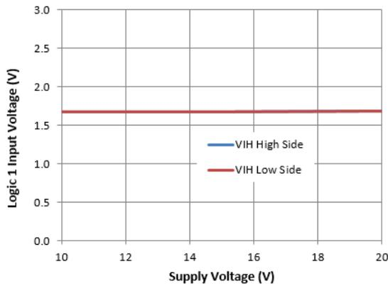
**Figure 19.** Logic 1 Input Voltage vs. Supply Voltage
