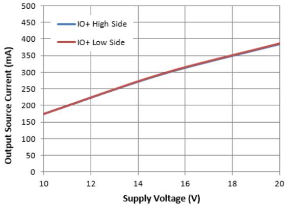
**Figure 15.** Output Source Current vs. Supply Voltage
