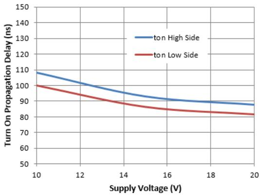
Figure 3. Turn-on Propagation Delay vs. Supply Voltage
