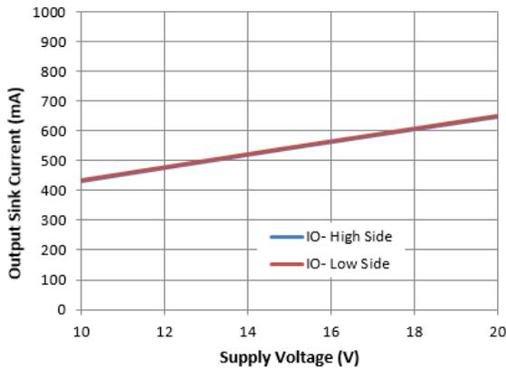
**Figure 17.** Output Sink Current vs. Supply Voltage
