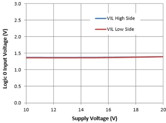
**Figure 21.** Logic 0 Input Voltage vs. Supply Voltage
