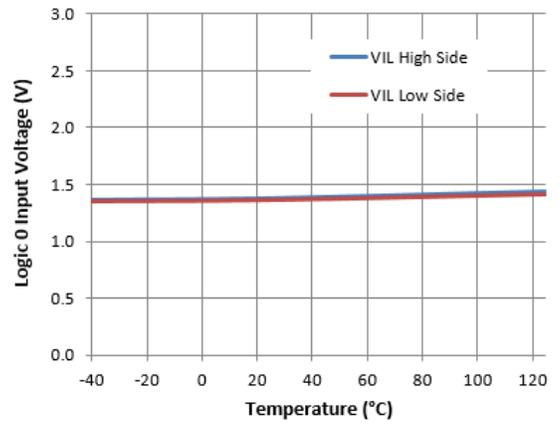
**Figure 22.** Logic 0 Input Voltage vs. Temperature
