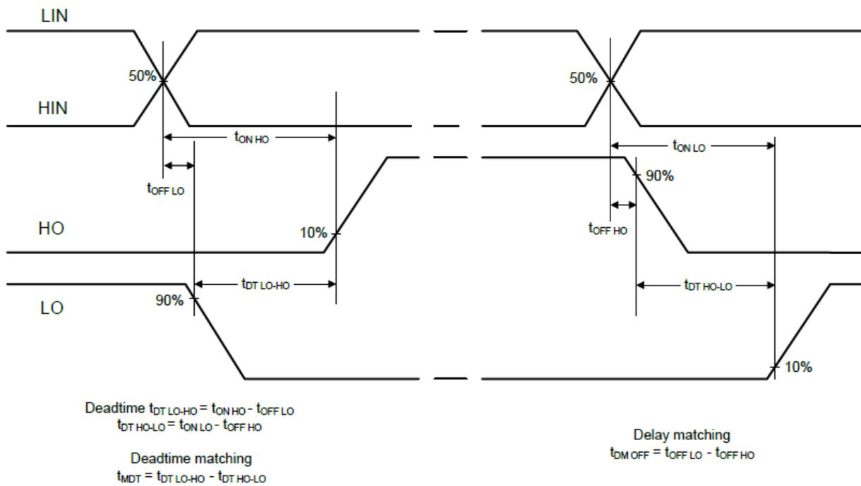
**Figure 2.** Switching Time Waveform Definition
