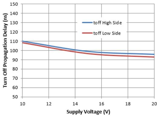
Figure 5. Turn-off Propagation Delay vs. Supply Voltage
