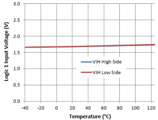
**Figure 20.** Logic 1 Input Voltage vs. Temperature
