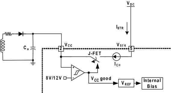
Figure 14. Startup Circuit
