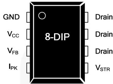
Figure 3. Pin Configuration
