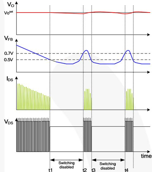
Figure 22. Burst-Mode Operation
