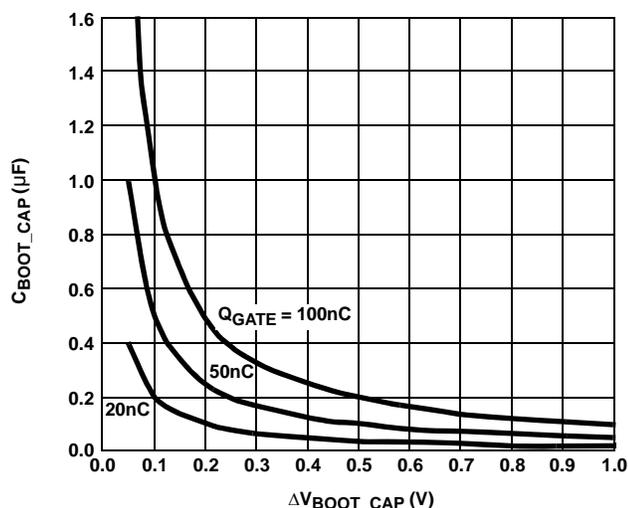
FIGURE 2. BOOTSTRAP CAPACITANCE vs BOOT RIPPLE VOLTAGE
